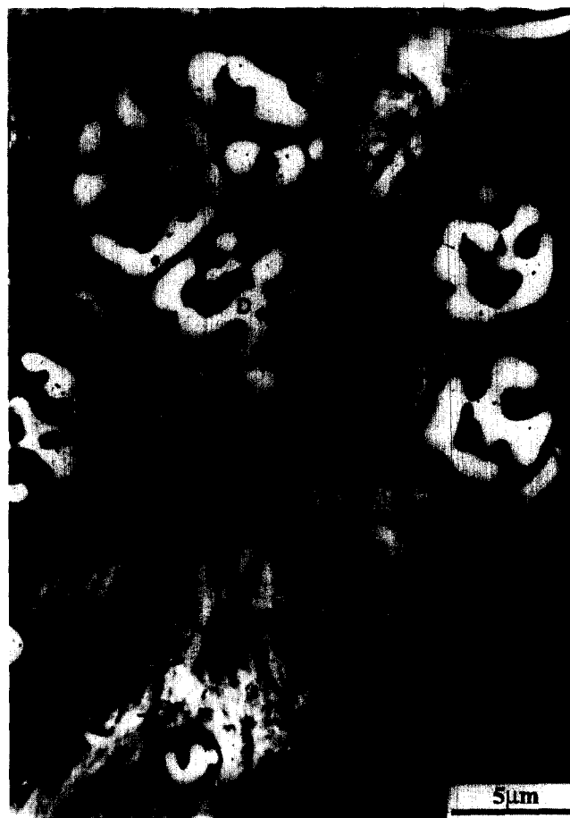
Figure 3 TEM micrograph of a PP/HDPE/PS/PMMA 60/20/10/10 blend (A = PP, B = HDPE, C = PS, D = PMMA)
