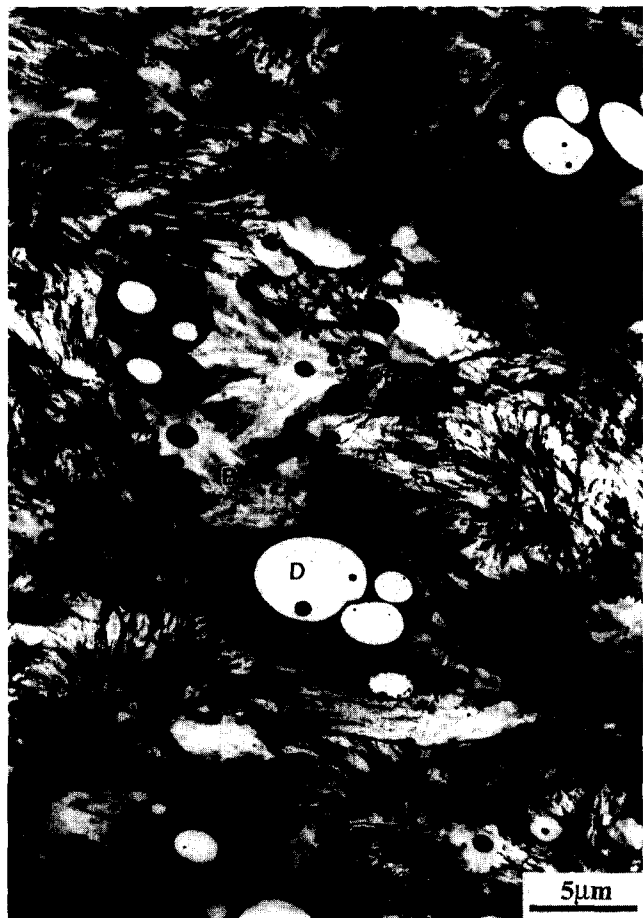
Figure 11 TEM micrograph of an HDPE/PP/PS/PMMA 65/20/10/5 blend (A = HDPE, B = PP, C = PS, D = PMMA)
