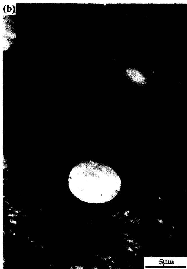
Figure 9 (a) TEM micrograph of an HDPE/PP/PS/PMMA 60/20/10/10 blend ( V_{\text{PP}}/V_{\text{PS}} = 2 ); (b) TEM micrograph of an HDPE/PP/PS/PMMA 75/5/10/10 blend ( V_{\text{PP}}/V_{\text{PS}} = 0.5 ) (A = HDPE, B = PP, C = PS, D = PMMA)
