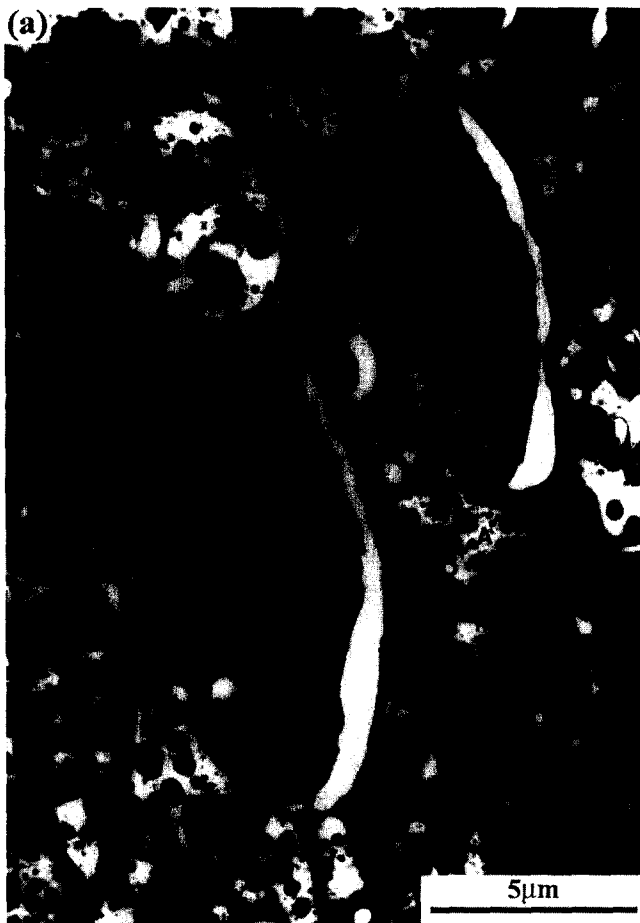
Figure 7 (a) TEM micrograph of a PMMA/PS/PP/HDPE 60/20/10/10 blend; (b) SEM micrograph of the fracture surface of a PMMA/PS/PP/HDPE 60/20/10/10 blend. The fracture surface was etched with cyclohexane (A = PMMA, B = PS, C = PP, D = HDPE)
