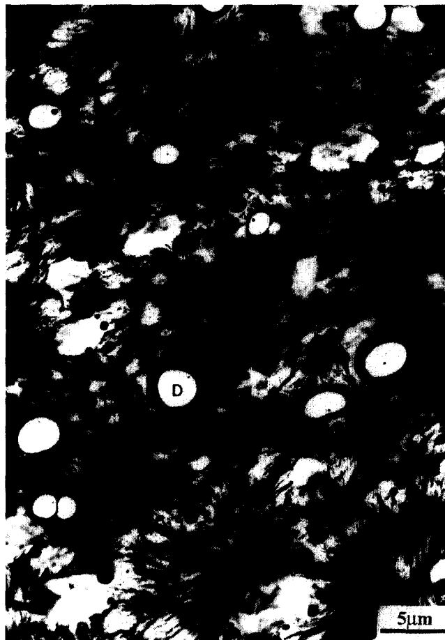
Figure 12 TEM micrograph of an HDPE/PP/PS/PMMA 65/20/10/5 blend containing 0.5% w/w S-E block copolymer (A = HDPE, B = PP, C = PS, D = PMMA)
