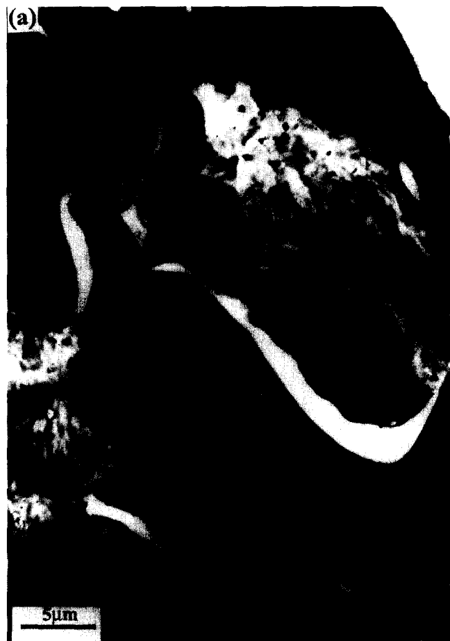
Figure 5 (a) TEM micrographs of a PS/PP/HDPE/PMMA 60/20/10/10 blend; (b) SEM micrograph of the fracture surface of a PS/PP/HDPE/PMMA 60/20/10/10 blend. The fracture surface was etched with a methanol/water mixture (A = PS, B = PP, C = HDPE, D = PMMA)
